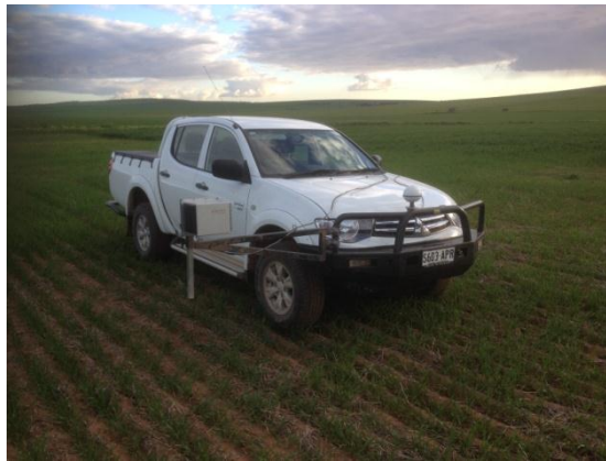
Above: The H-Sensor mounted to the ute for mapping and collecting images of the crop and weeds.
