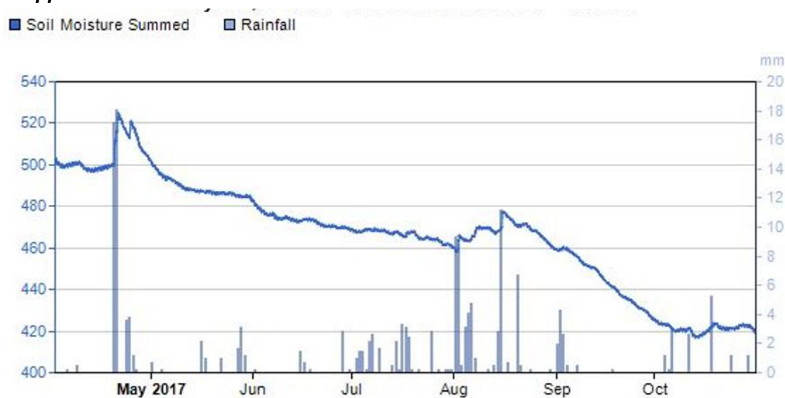
Figure 2. Summed soil moisture chart showing total soil moisture in the soil profile (line) and rainfall (columns) during the 2017 growing season (April-October) at a site that was planted to wheat in 2017.
