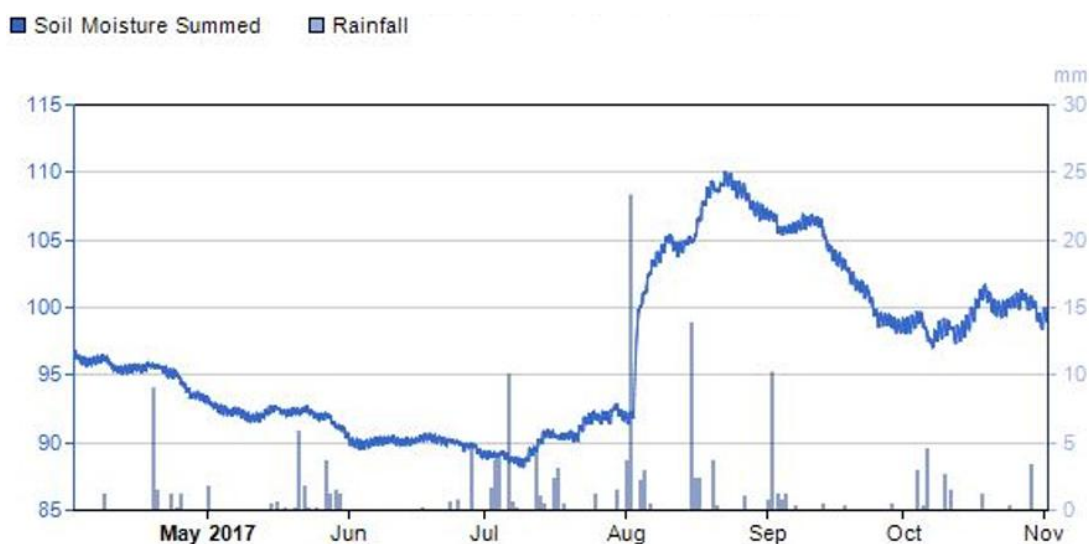
Figure 3. Summed soil moisture chart showing total soil moisture in the soil profile (line) and rainfall (columns) during the 2017 growing season (April-October) at a site that was a regenerated pasture in 2017.
