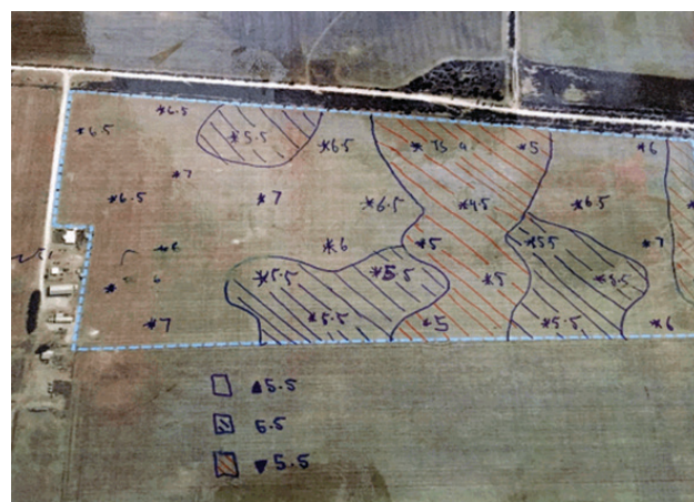
Figure 2. Luke's manual pH map. Produced using field pH kit and aerial photo, March 2016.
