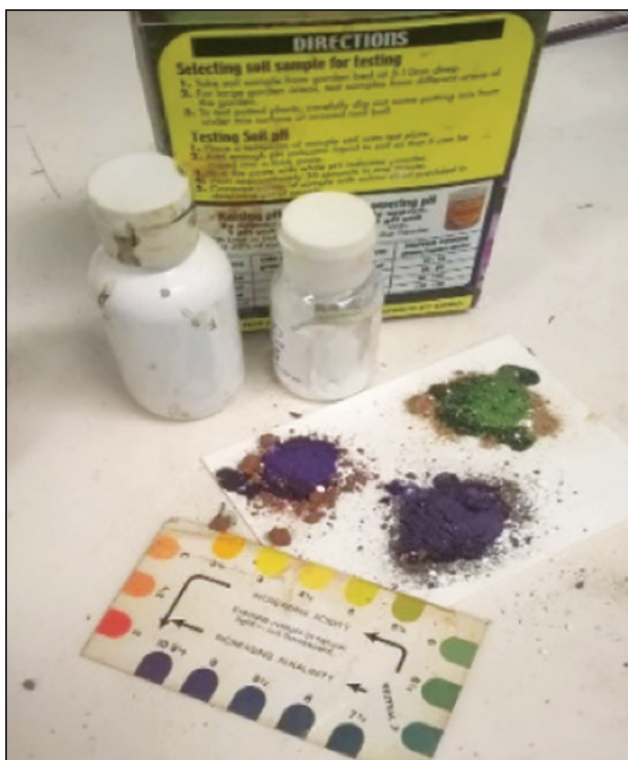
Figure 2. Field kits give soil pH values which are approximate to pH(water).
