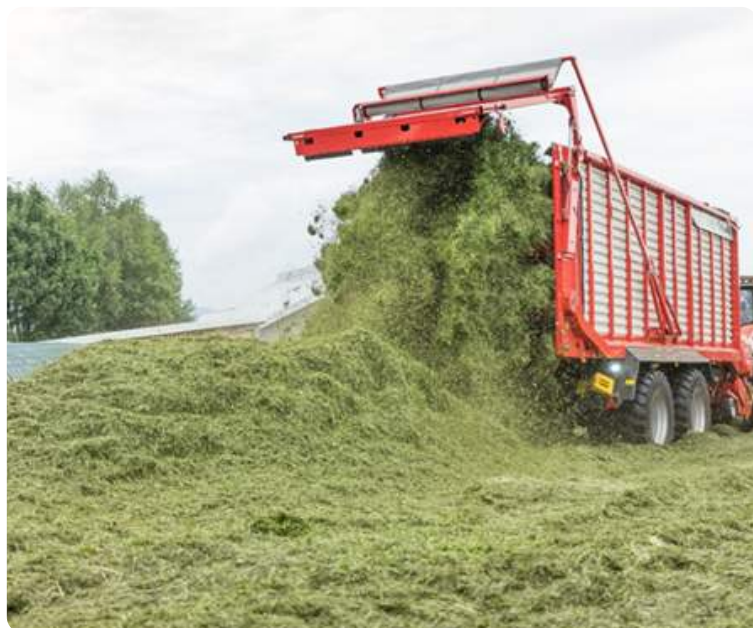
Figure 4. Forage wagon unloading silage into a bunker. The forage wagon can also be used to feed out silage. Check carefully for rust and wear/tear if purchasing second hand.
