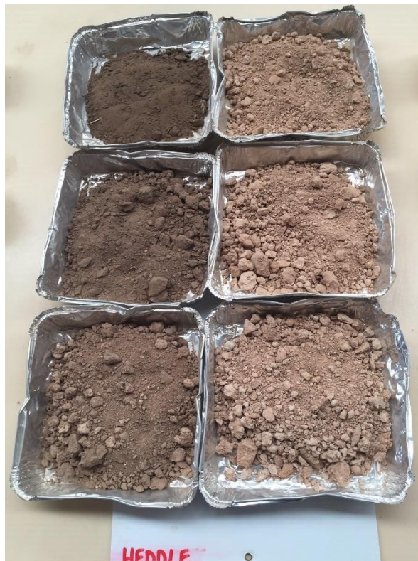
Photo: LHS (top tray) 0-10 cm, middle 10-30 cm, bottom 30-60 cm. RHS (top tray) 60-90 cm, middle 90-120 cm, bottom 120-150 cm.
