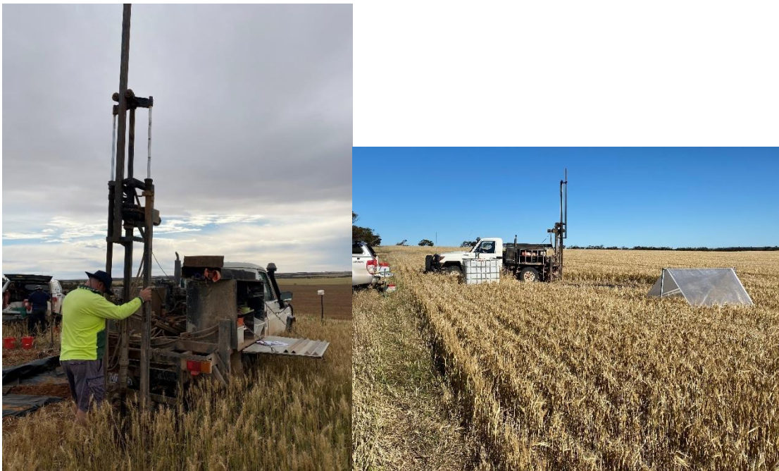
SARDI drill rig used to collect soil chemistry samples and rain out shelter to collect CLL soil samples.
