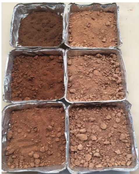
Photo: LHS (top tray) 0-10 cm, middle 10-30 cm, bottom 30-60 cm. RHS (top tray) 60-90 cm, middle 90-120 cm, bottom 120-150 cm.
