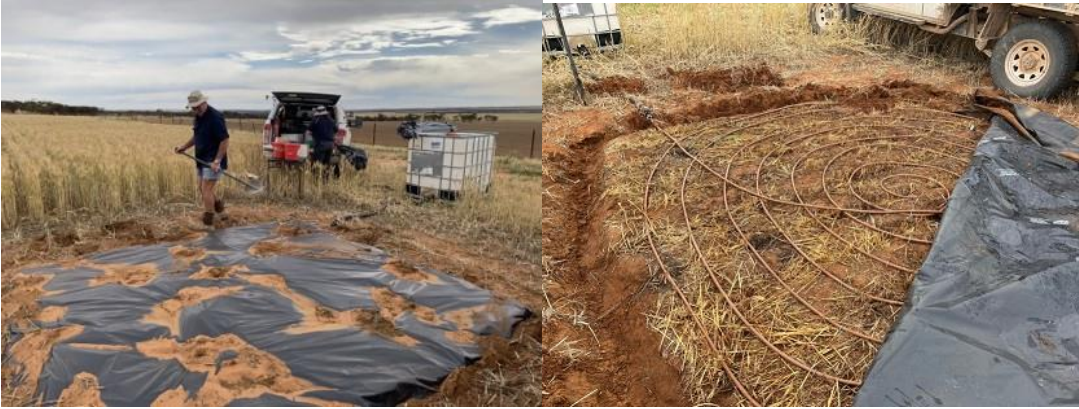
Buckleboo site covered with plastic to prevent evaporation for DUL and bulk density. Circular layout of dripper hose for wetting up soil profiles.
