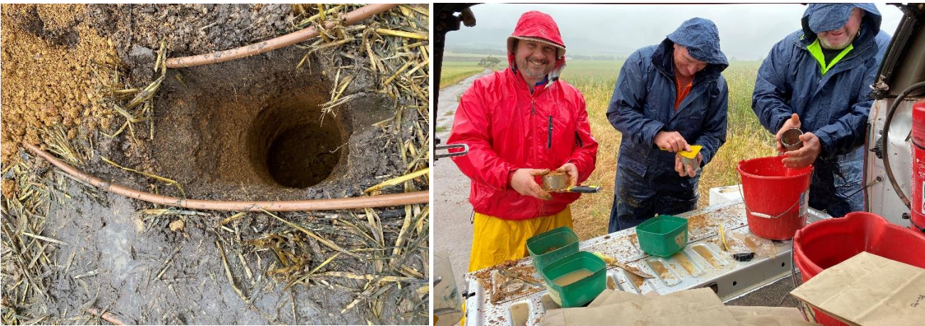
Sampling hole after bulk density sample taken using slide hammer and paring back soil samples to collect bulk density and DUL.
