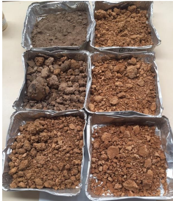
Photo: LHS (top tray) 0-10 cm, middle 10-30 cm, bottom 30-60 cm. RHS (top tray) 60-90 cm, middle 90-120 cm, bottom 120-150 cm.
