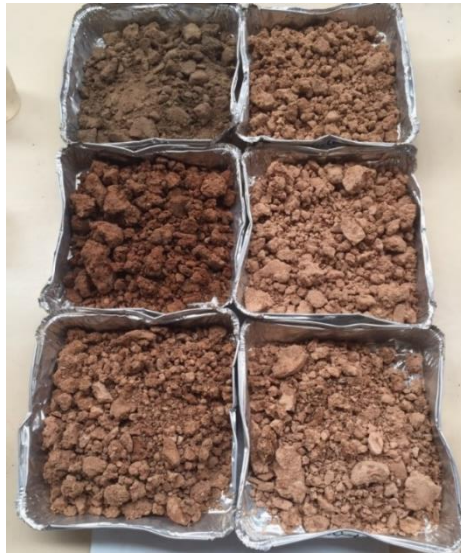
Photo: LHS (top tray) 0-10 cm, middle 10-30 cm, bottom 30-60 cm. RHS (top tray) 60-90 cm, middle 90-120 cm, bottom 120-150 cm.
