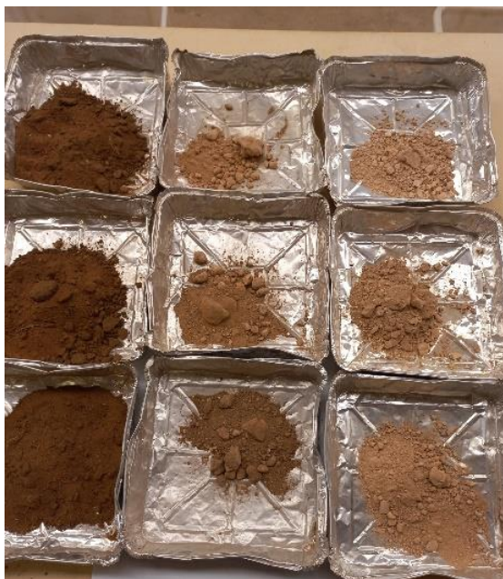
Photo: LHS (bottom tray) 0-10 cm, middle 10-20 cm, top 20-30 cm. Middle (bottom tray) 30-40 cm, middle 40-50 cm, top 50-60 cm. RHS (bottom tray) 60-80 cm, middle 80-100 cm, top 100-120 cm.
