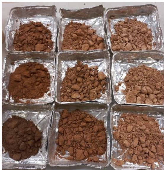
Photo: LHS (bottom tray) 0-10 cm, middle 10-20 cm, top 20-30 cm. Middle (bottom tray) 30-40 cm, middle 40-50 cm, top 50-60 cm. RHS (bottom tray) 60-80 cm, middle 80-100 cm, top 100-120 cm.
