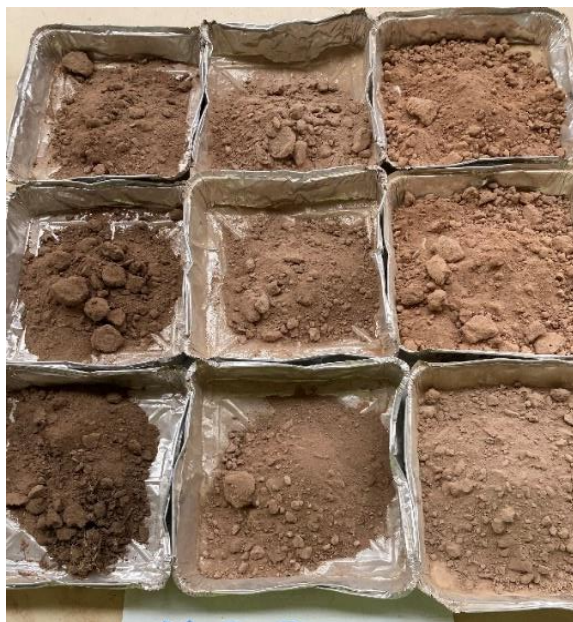
Photo: LHS (bottom tray) 0-10 cm, middle 10-20 cm, top 20-30 cm. Middle (bottom tray) 30-40 cm, middle 40-50 cm, top 50-60 cm. RHS (bottom tray) 60-80 cm, middle 80-100 cm, top 100-120 cm.
