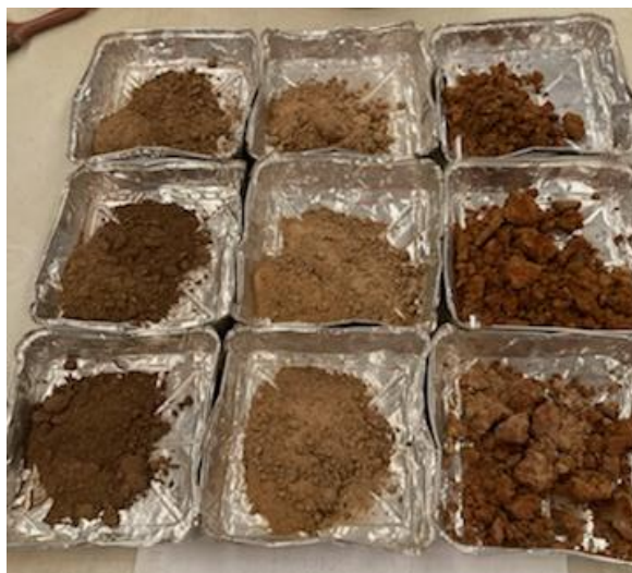
Photo: LHS (bottom tray) 0-10 cm, middle 10-20 cm, top 20-30 cm. Middle (bottom tray) 30-40 cm, middle 40-50 cm, top 50-60 cm. RHS (bottom tray) 60-80 cm, middle 80-100 cm, top 100-120 cm.
