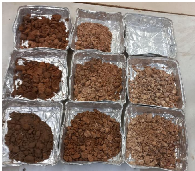
Photo: LHS (bottom tray) 0-10 cm, middle 10-20 cm, top 20-30 cm. Middle (bottom tray) 30-40 cm, middle 40-50 cm, top 50-60 cm. RHS (bottom tray) 60-80 cm, middle 80-100 cm, top 100-120 cm.
