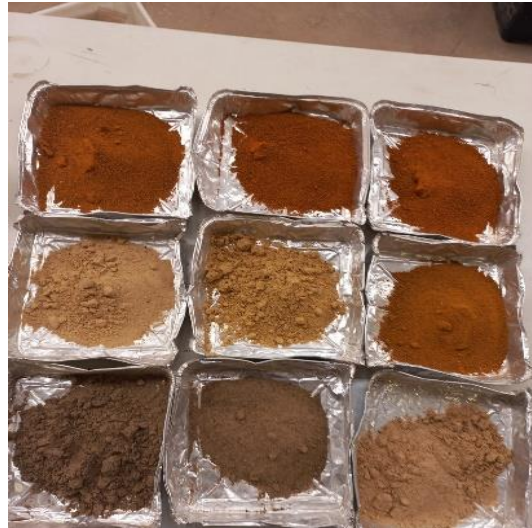
Photo: LHS (bottom tray) 0-10 cm, middle 10-20 cm, top 20-30 cm. Middle (bottom tray) 30-40 cm, middle 40-50 cm, top 50-60 cm. RHS (bottom tray) 60-80 cm, middle 80-100 cm, top 100-120 cm
