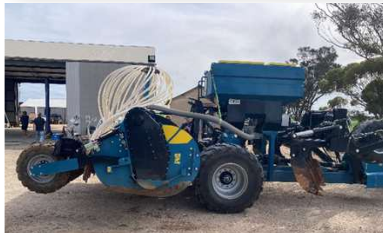
Tim's Imants spader with deep ripping boots at front and fitted with seed box. [Source: Tim Polkinghorne]
